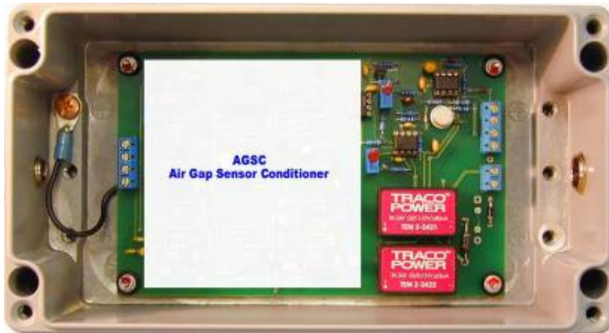
Figure 24. AGS Signal Conditioner unit enclosure with cable inlets (CAB) (before S/N 144701)
