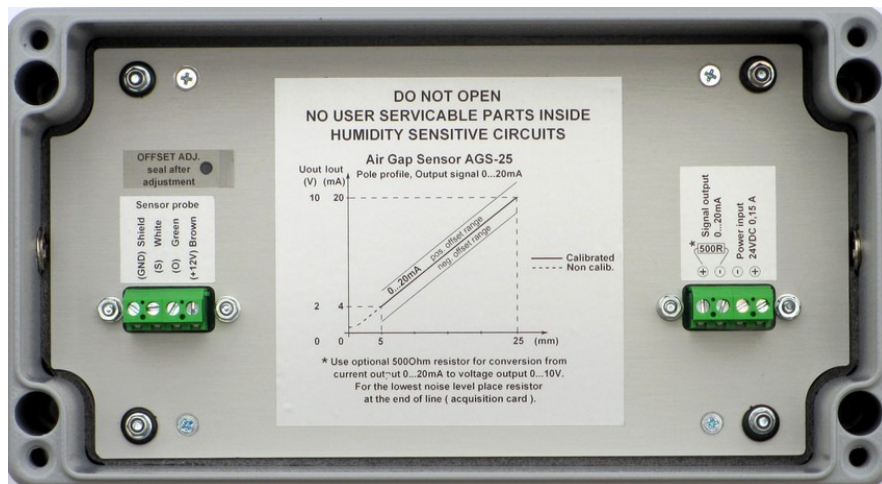
Figure 25. AGS Signal Conditioner unit enclosure with cable inlets (CAB) (after S/N 144701)
