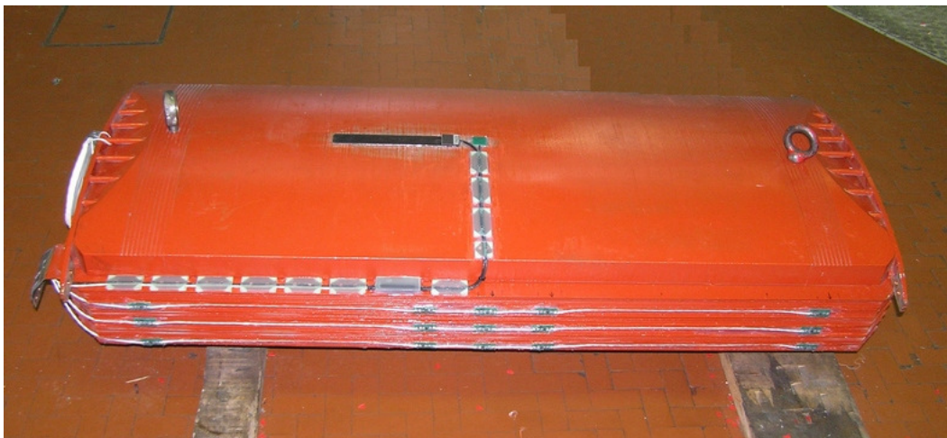
Figure 32. AGSP sensor probe installed at rotor pole (AGSP sensor pictured next to Magnetic field sensor in the middle of rotor pole)
