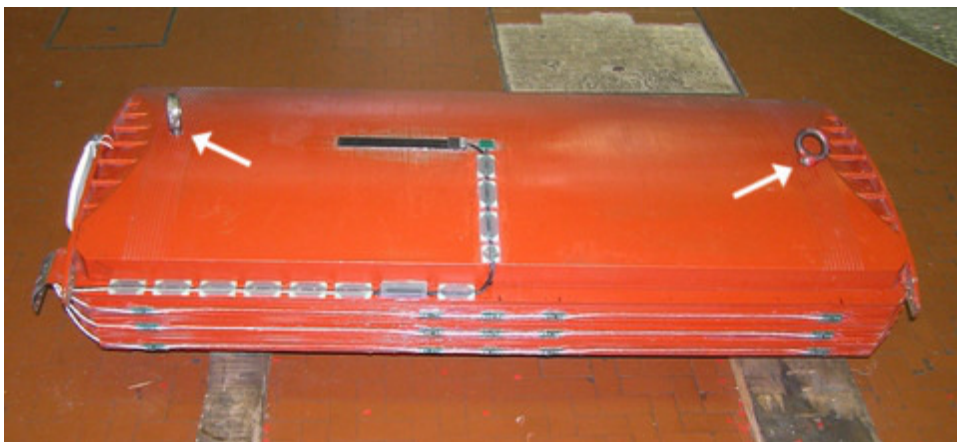
Figure 5: Rotor pole, arrow showing positions of pole lifting hoist attachments
